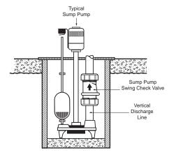
General Installation Information: Sump Pump Swing Check Valves may be installed in either vertical up-flow (see illustration) or horizontal positions on pump discharge line. Check valves MUST be installed with the valve's FLOW arrow pointing in the direction of the flow. In horizontal installations, the designated side must be positioned "up". Do Not install Check Valve upside down.
