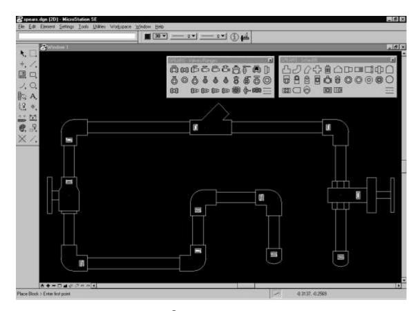
**Completed SPEARS<sup>®</sup> 2D Process Pipe and Fitting Layout**
