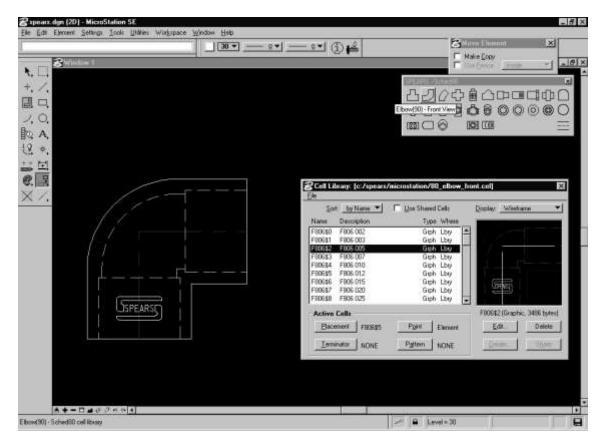
Placing SPEARS<sup>®</sup> Fitting Cell in Microstation<sup>®</sup>
