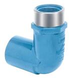
Designed for use where over tightening of threads is a problem. This unique precompression design compensates for expansion forces generated from tapered pipe thread joint make-up. Radial stress is reduced in normal installations and contained in severe over tightening situations. Available as an individual component.
