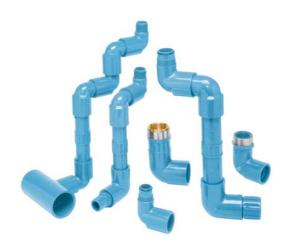
Spears® EverTUFF® TURF™ Swing Joint RiserAssemblies are precision engineered for use in turf and landscape irrigation applications. Molded to a strong Schedule 80+ design from high quality PVC, Spears® Swing Joint Riser Assemblies offer full 360° adjustment on three planes, and are available in a variety of inlet/outlet combinations in 1", 1-1/4" and 1-1/2" ASTM IPS; 1", 1-1/4" and 1-1/2" BSP Threaded; 32mm, 40mm and 50mm DIN; and 25mm, 32mm, and 40mm JIS.
