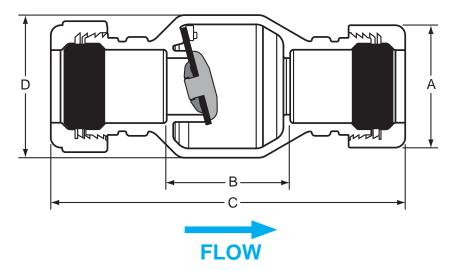
**WARNING:** The compression joints provide a positive seal but do not restrain pipe from thrust and movement under pressure. Use of compression joint requires blocking of connecting pipe to prevent any movement. Failure to do so can result in system failure or severe personal injury. Use in cold water/fluid applications only.
