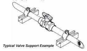
**CAUTION:** All valve connectors and connecting pipe should be inspected for any breaking, chipping, gouging or other visible damage before proceeding. All joining components must be clean and dry. All valves and pipe shall be removed from their packaging or containers and exposed to the environment for a minimum of one hour in order to thermally balance all components. Installation temperatures should be between 40°F and 110°F.
